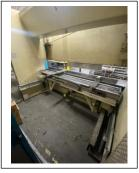
Main MotorTBA KwElectrical Supply400v | 50Hz | 3PhDimensions 'approx'<br/>without front support arms4150 [L] x 2000 [W] x 2900 [H]Machine weight 'approx'11,500 KgTop & Bottom ToolingNO TOOLING
