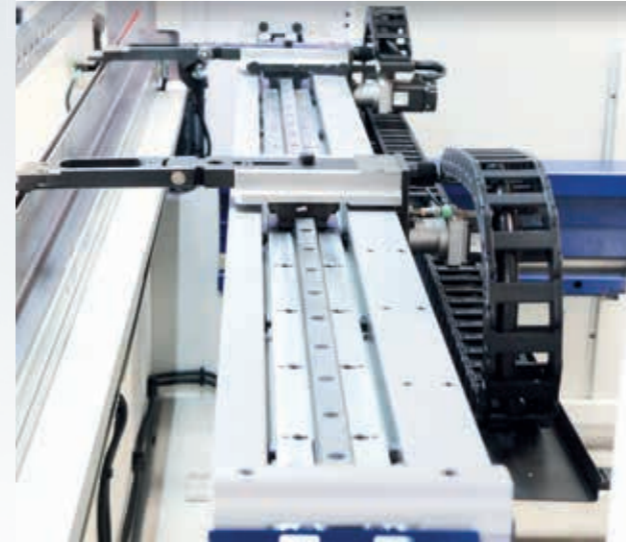
X travel 750mm, R travel 250mm - X5 travel 200mm ( \pm 100 mm) Z1, Z2 travel up to back gauge length
