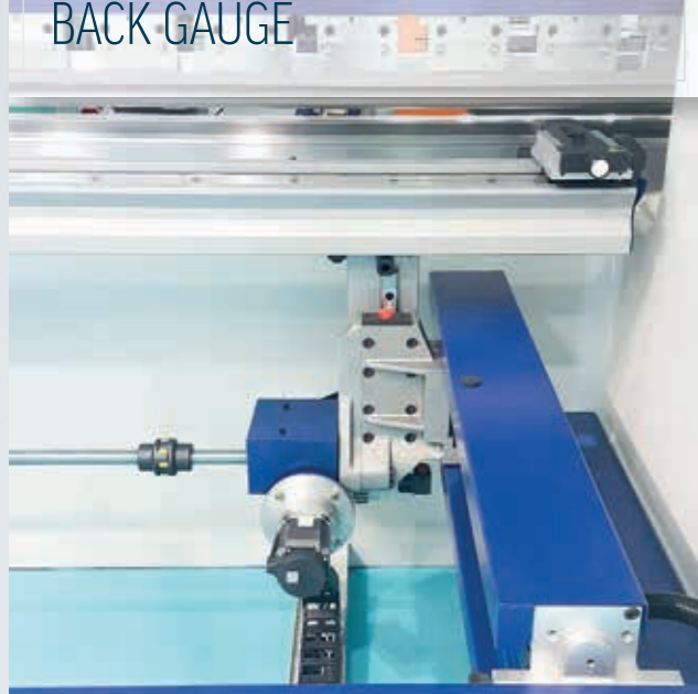
X travel 750mm, R travel 250mm - Reinforced R Axis with linear sliding
