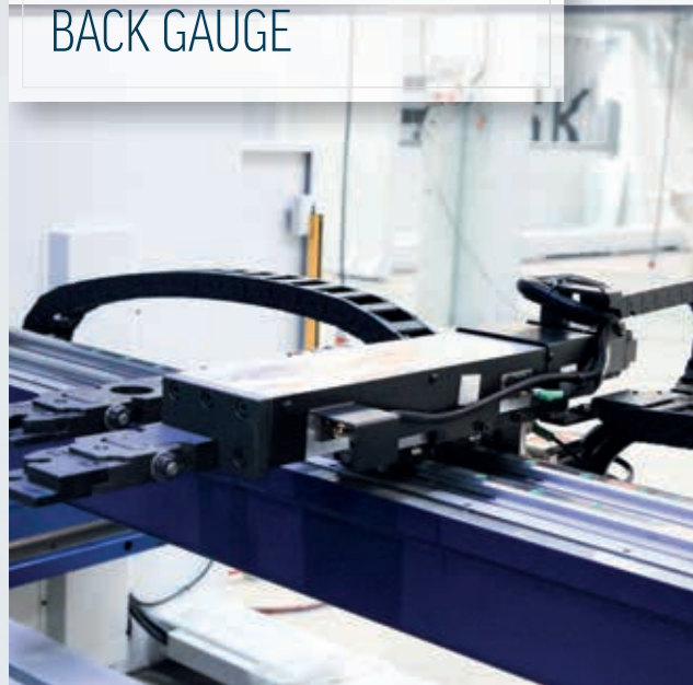
X travel 750mm, R travel 250mm - Z1, Z2 travel up to back gauge length
